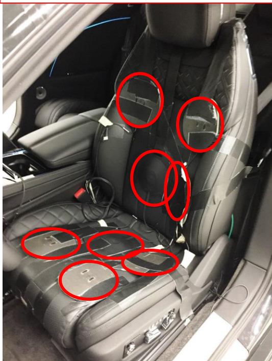
Redundant Vibration Receiver Points
