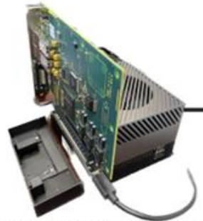
NVIDIA Jetson Orin Developer Kit with one of Concurrent Real-Time's FPGA-based Intelligent I/O Boards
