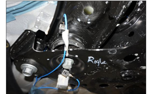
VPT measurement on the vehicle on active and passive side of the mount
