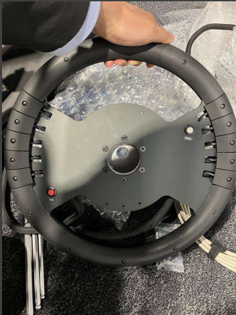
Steering Wheel Grip Force Sensor Measurement of the driver's tension level and research on its use as an interactive device.
