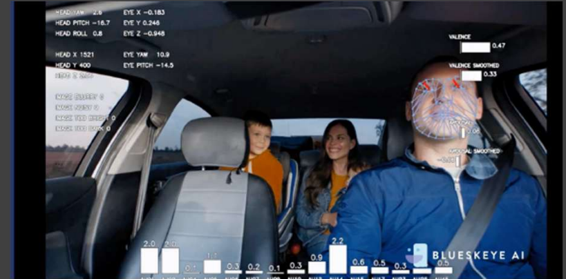
Blueskeye AI B-Automotive Capture facial skin movements on video and analyze them with AI to estimate the driver's feeling.
