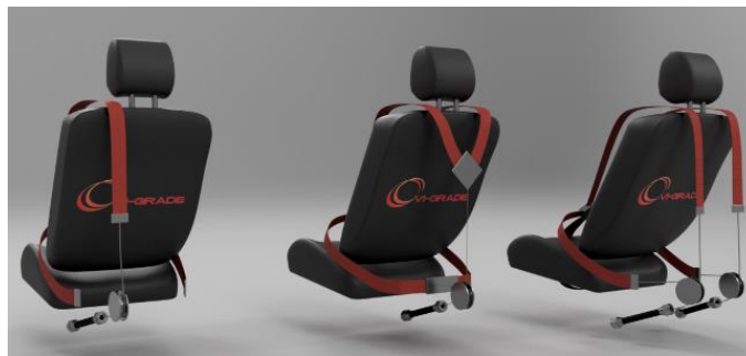
Fig. 4: Active seat and active belts system
