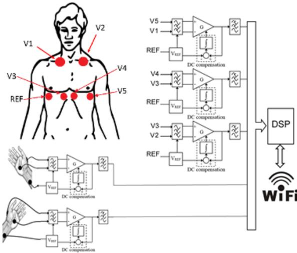
Figure 1: Sensor block diagram
