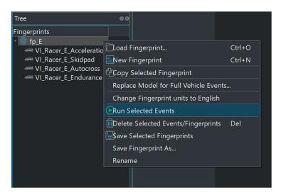
Alternatively, to run an individual simulation, you can right click directly on a single event.
