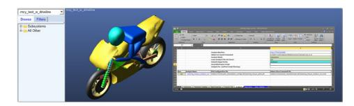
• Path Compensation event supports vdf\_template: the user has the possibility to submit a path compensation analysis using a vdf template in which he can define his own custom settings for VI-Rider.
