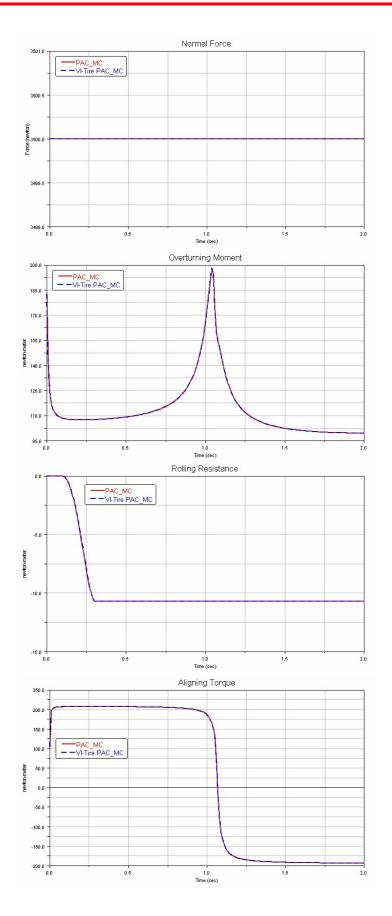
Some differences may appear at extreme inclination angles when the contact patch exceeds the limits of the supplied tire profile. When this condition occurs VI-Tire prints a warning in the ADAMS message file:
