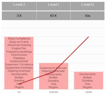
Based on single switch, accessible in the system parameter tree, the user can define which fidelity level to use for a simulation task. The first application of this technology is in the context of the Press Maneuver event: using a less refined, but faster, model for the initial steps of the optimization process, grants an overall reduction in computation time with results equivalent to the usage of the full model for the entire process.
