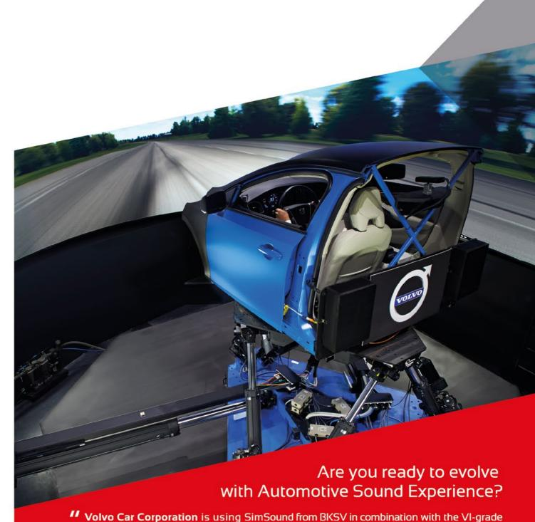
DiM150 dynamic driving simulator for Vehicle Dynamics and ADAS assessments from early concept phase and throughout the development process. SimSound helps to create an immersive enrironment around the driver - ultimately helping the driver to perform as if he/she was driving a physical car - ensuring that we can perform high quality Driver-in-the-Loop testing.
